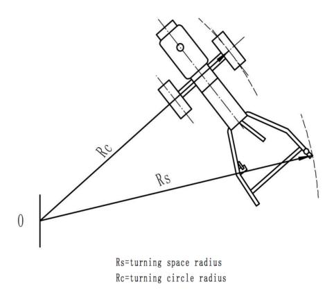
Fig 1: The measurement of radius of turning circle and turning space.
